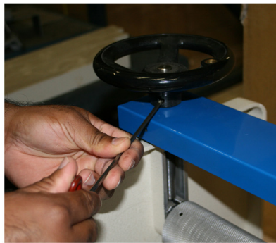
2. Loosen both set screws at the base of the handwheel.
